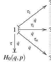
**Fig. 2** Attachment of a multiple image feature bonds. Each image feature contributes an effort  $\tau_i$  to the 1-junction that couples with the flow  $\dot{q}$  of the mechanical system. These efforts sum to produce the IBVS control action. The question marks indicate that this part of the bondgraph remains to be defined.
