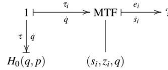
**Fig. 3** Modulated transformer to relate image flow  $\dot{s}_i$  with the flow  $\dot{q}$  at the 1-junction.
